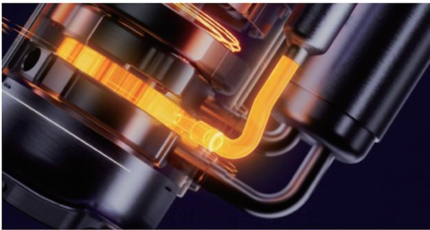
When the system operates under extreme cold conditions, the compressor supplies mid-temperature vapor to increase the total amount of compressed refrigerant, enhancing the heat performance.
