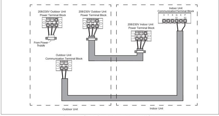
Figure 28. Single-Zone Wiring 36K and 48K Only
