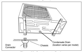
Figure 22. Condensate Drain
