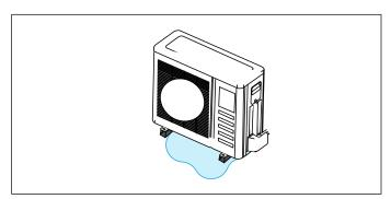
Figure 18. Avoid Defrost Water Ice Hazard
