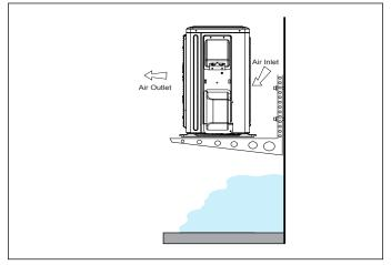
Figure 16. Outdoor Unit on Brackets above Snow Line
