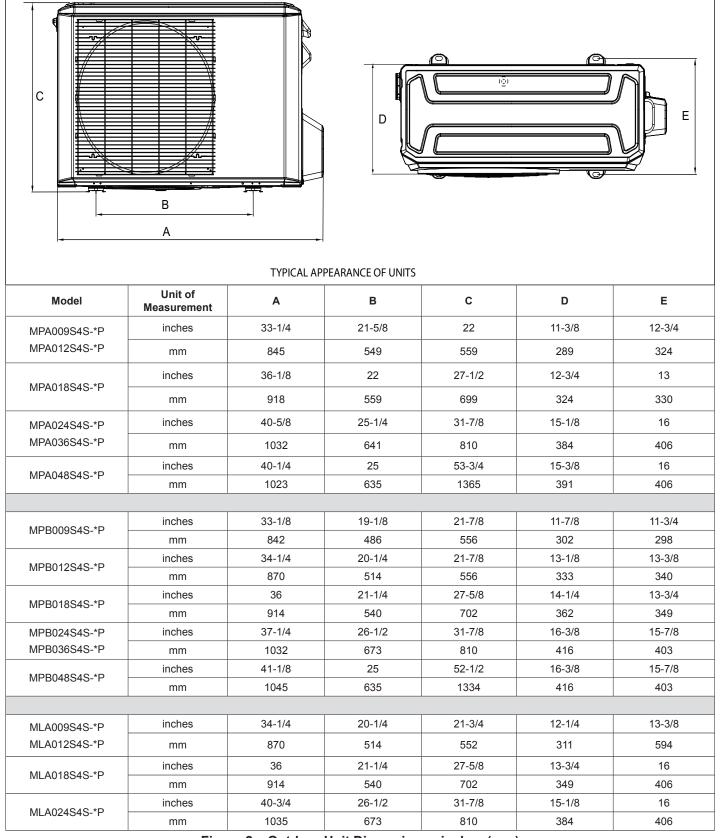
Figure 2. Outdoor Unit Dimensions - inches (mm)
