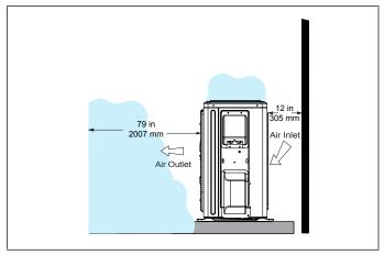
Figure 17. Outdoor Unit Air Flow Obstructed by Snow
