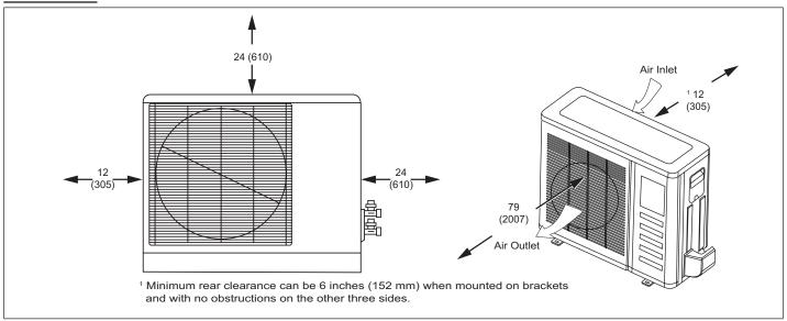
Figure 4. Outdoor Unit Clearances - Inches (mm)
