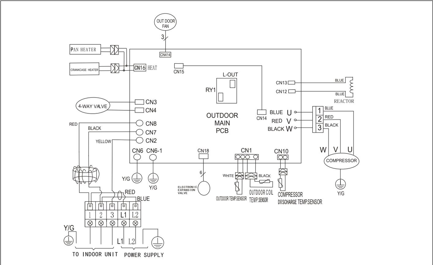
Figure 33. 208/230V MPA018S4S-\*P Outdoor Unit Wiring Diagram
