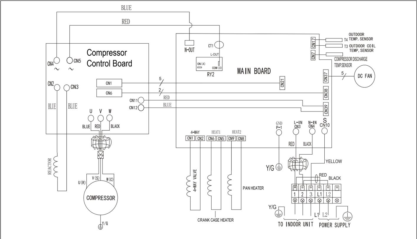
Figure 34. 208/230V MPA024S4S-\*P Outdoor Unit Wiring Diagram
