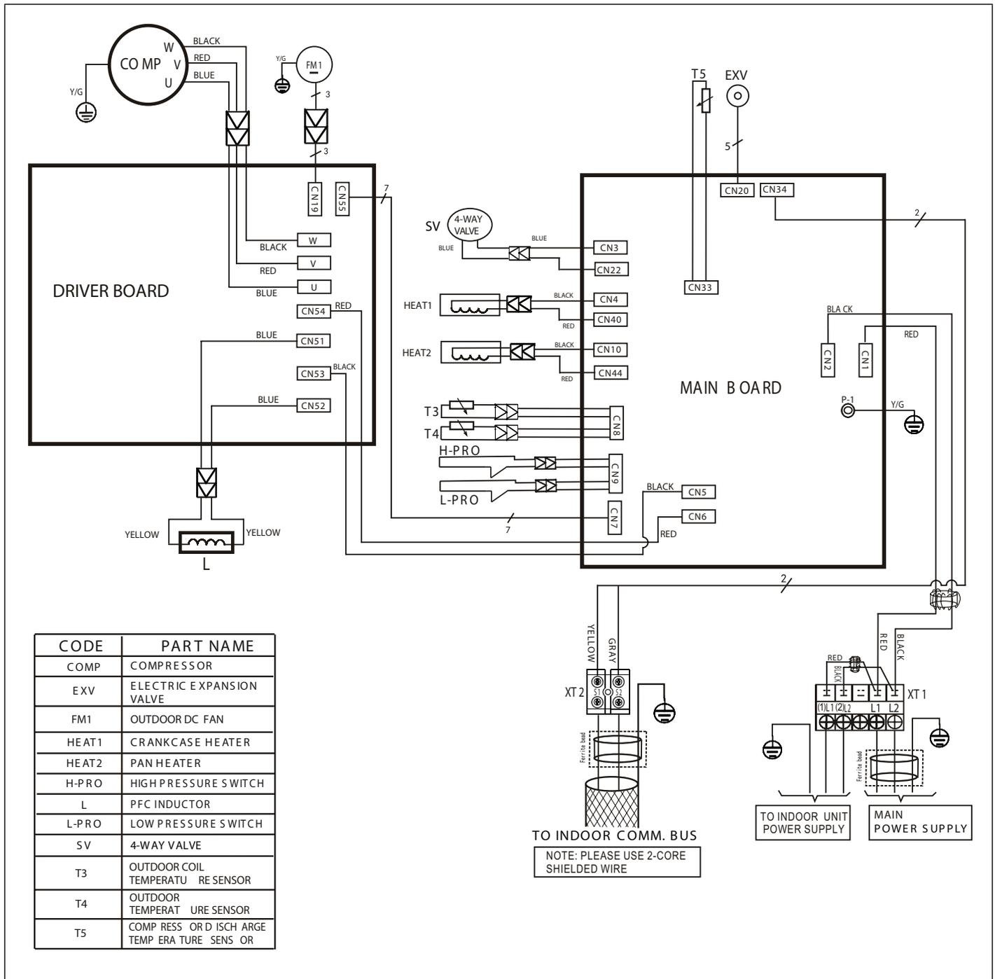
Figure 39. 208/230V MPB036S4S-\*P Outdoor Unit Wiring Diagram
