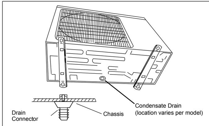
Figure 22. Condensate Drain
