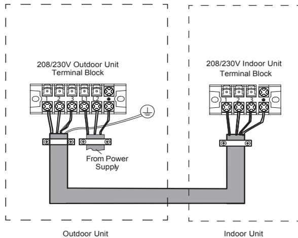
Figure 27. Single-Zone Wiring 24K and Below
