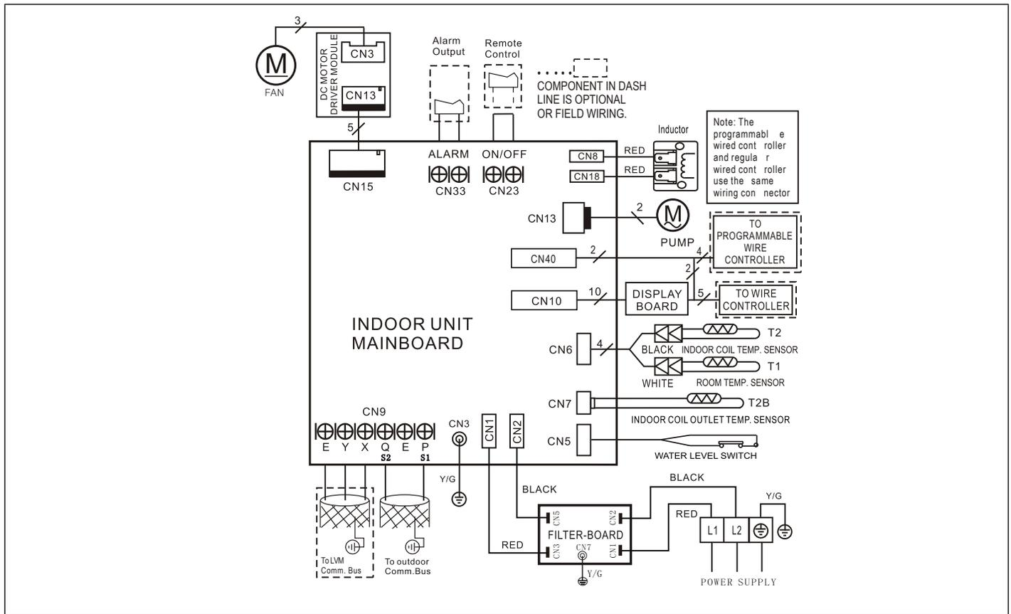
Figure 31. MMDA036S4-\*P & MMDA048SA-\*P Ducted Units Wiring Diagram
