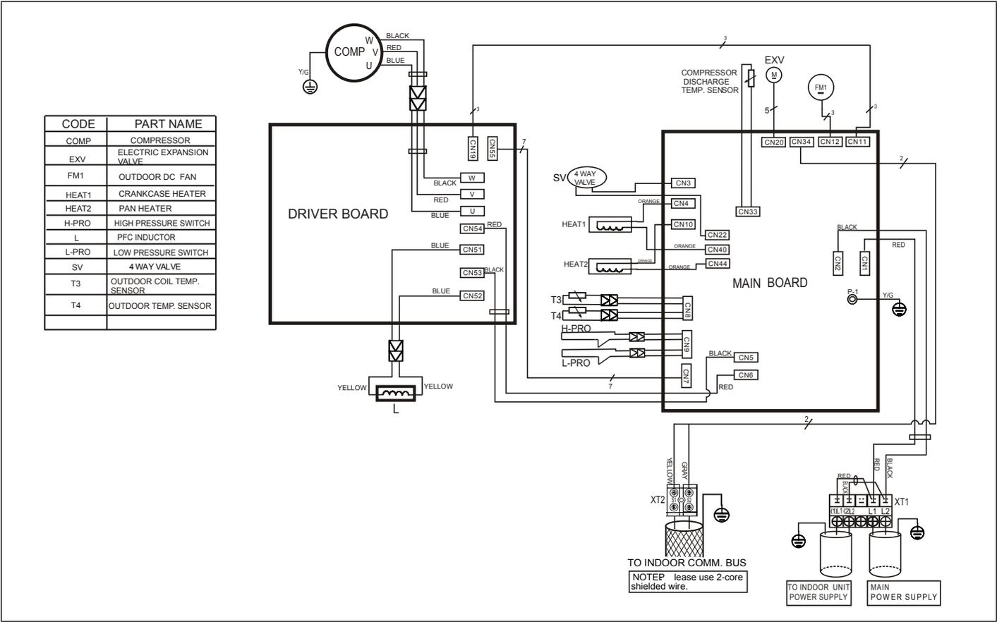
Figure 35. 208/230V MPA036S4S-\*P Outdoor Unit Wiring Diagram
