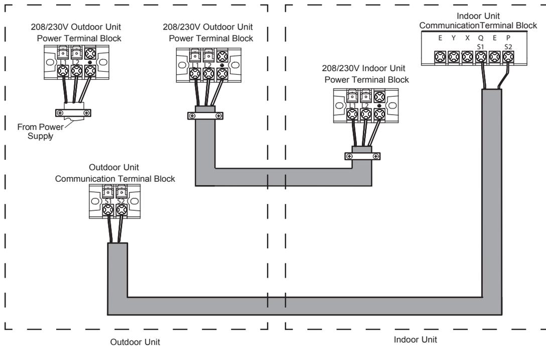
Figure 28. Single-Zone Wiring 36K and 48K Only
