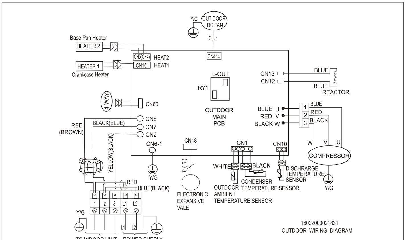
Figure 41. 208/230V MLA009, 012 and 018S4S-\*P Outdoor Unit Wiring Diagram
