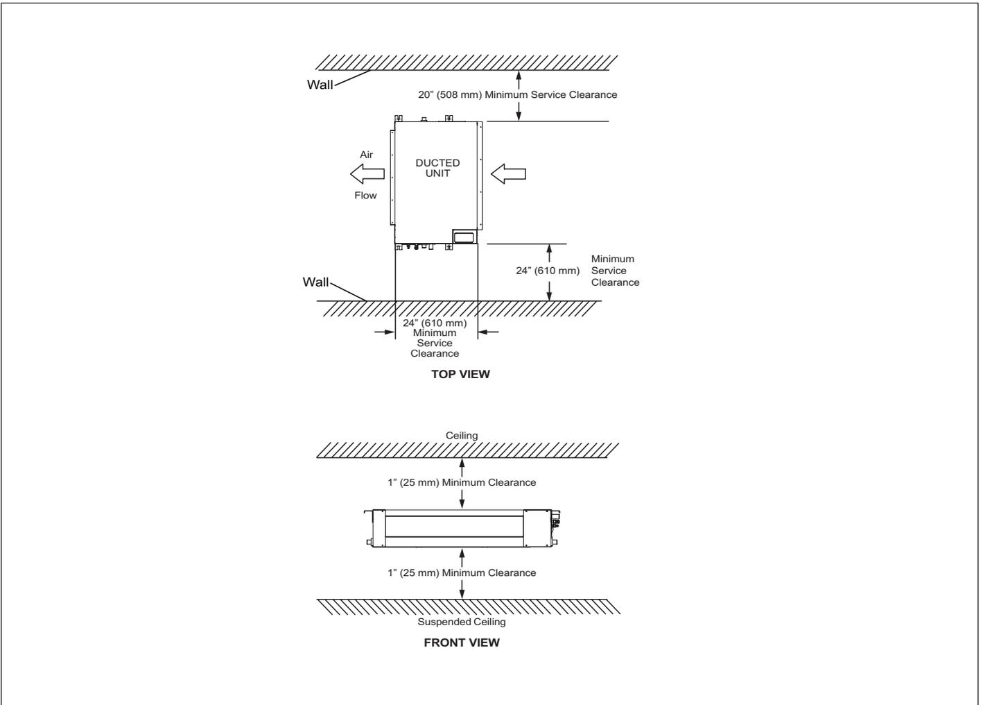
**Figure 5. Indoor Unit Clearances - Inches (mm)**
