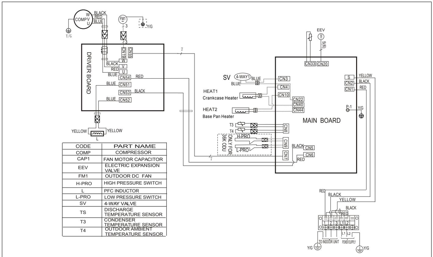
Figure 42. 208/230V MLA024S4S-\*P Outdoor Unit Wiring Diagram
