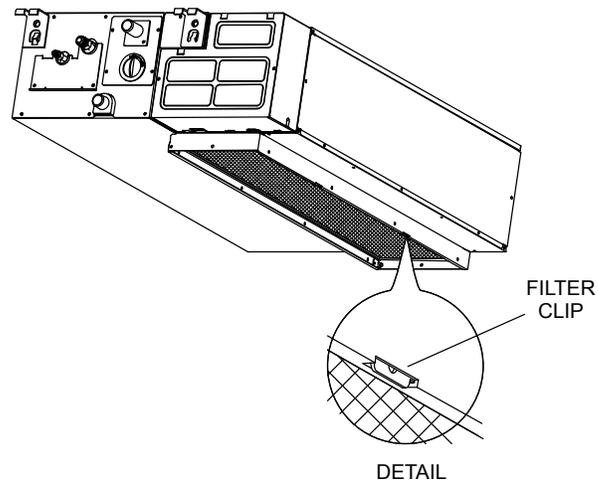
**Figure 9. Field-Relocation of Return Air Filter (Typical) - Bottom Return Air**
