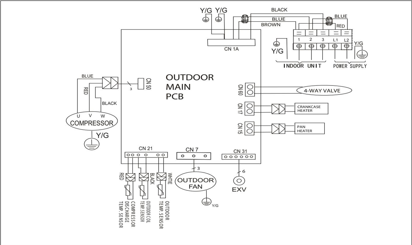
Figure 37. 208/230V MPB009S4S-\*P and MPB012S4S-\*P Outdoor Unit Wiring Diagram
