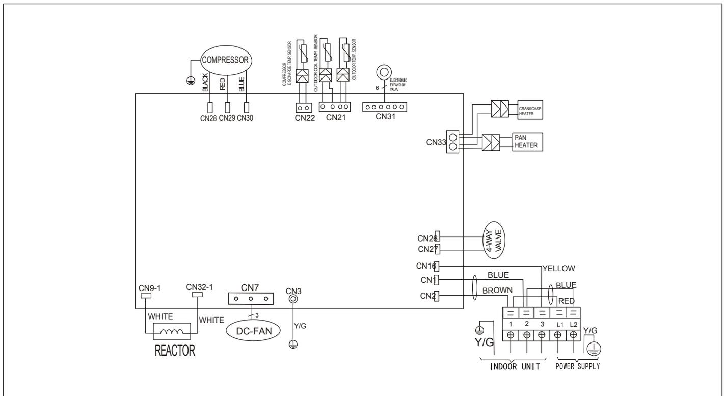
Figure 32. 208/230V MPA009S4S-\*P and MPA012S4S-\*P Outdoor Unit Wiring Diagram
