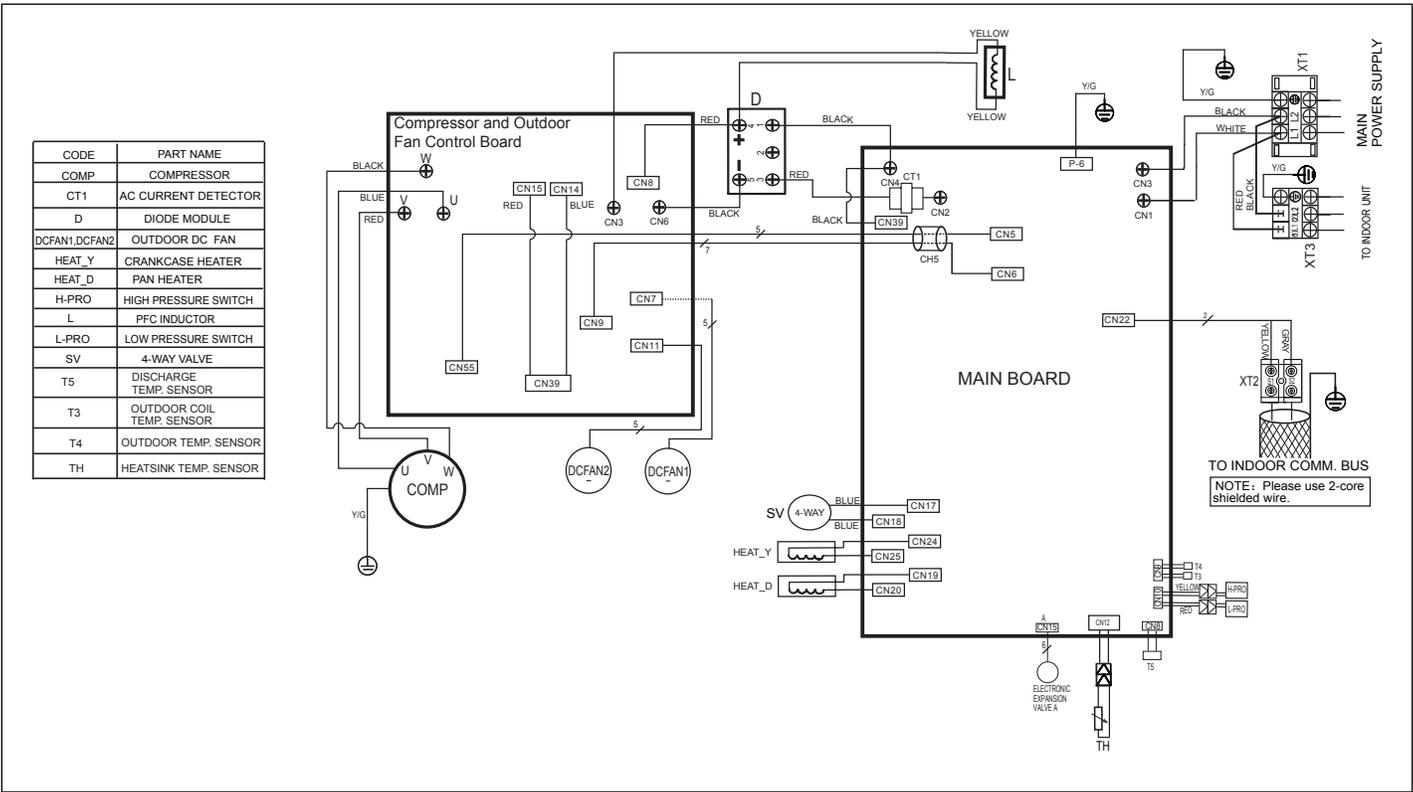
Figure 36. 208/230V MPA048S4S-\*P Outdoor Unit Wiring Diagram
