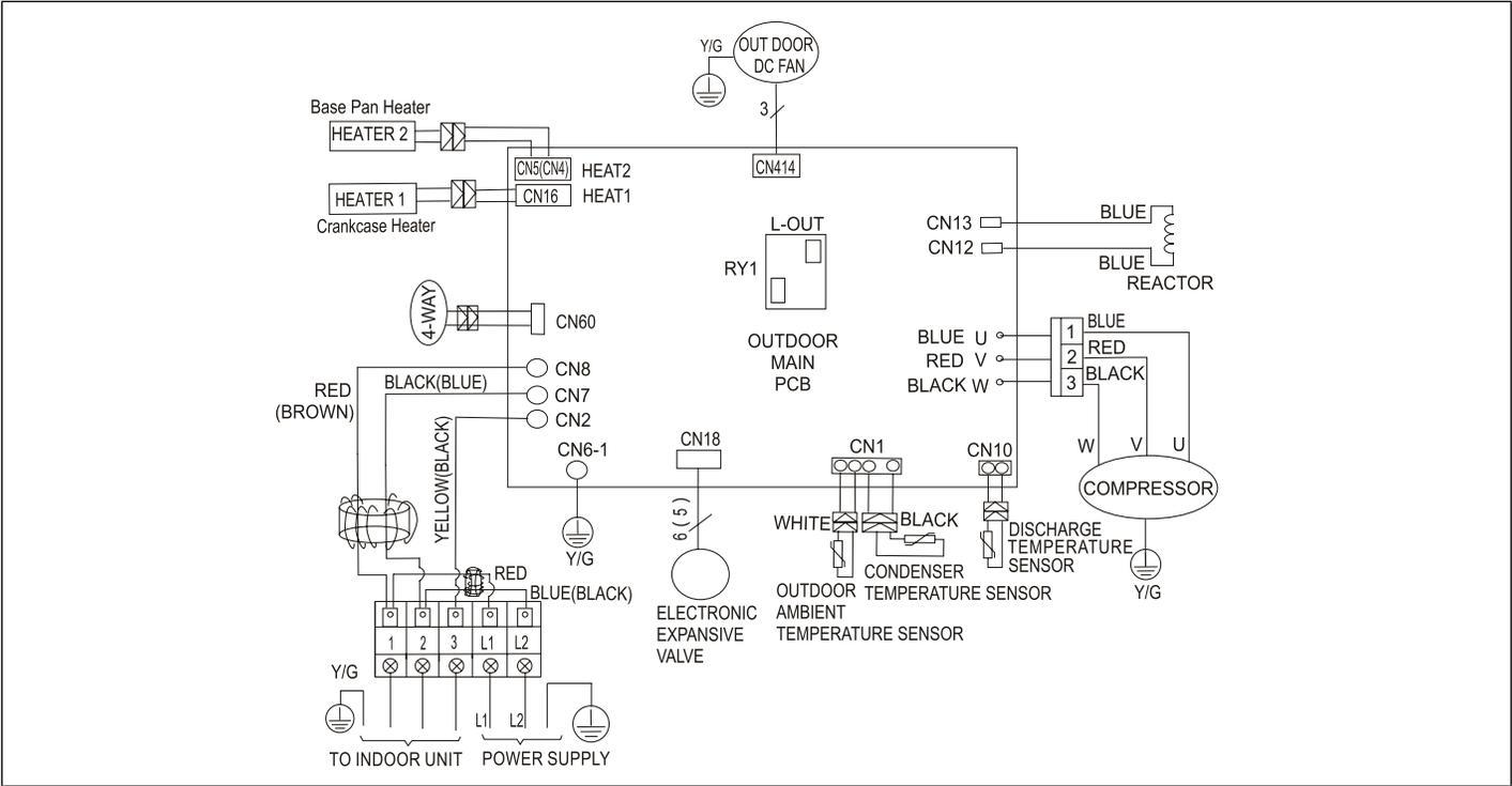
Figure 38. 208/230V MPB018S4S-\*P and MPB024S4S-\*P Outdoor Unit Wiring Diagram
