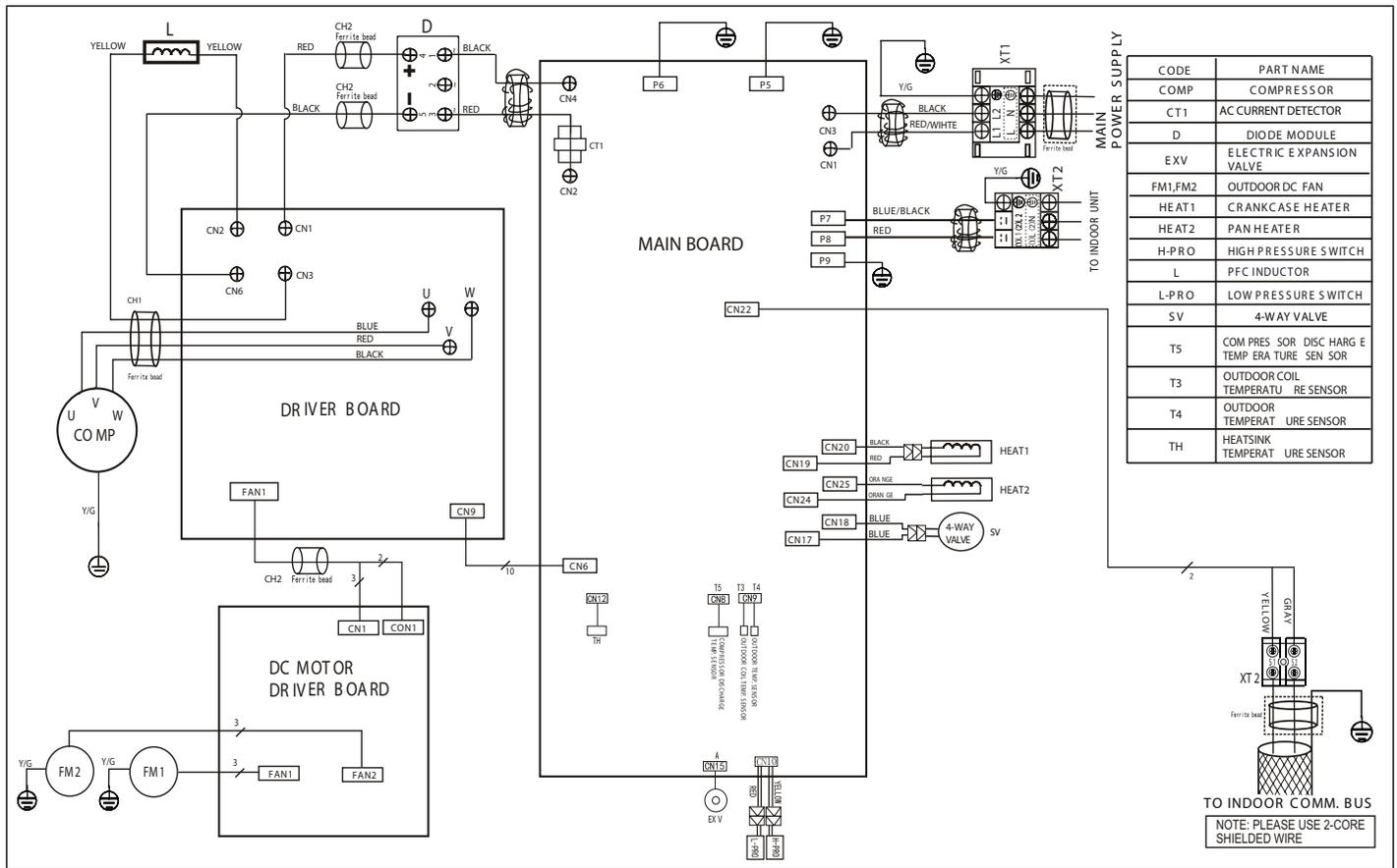
Figure 40. 208/230V MPB048S4S-\*P Outdoor Unit Wiring Diagram
