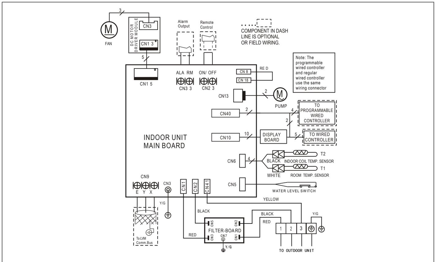
Figure 30. MMDA024S4-\*P Ducted Units Wiring Diagram
