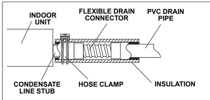
Figure 10. Condensate Gravity Drain Option
