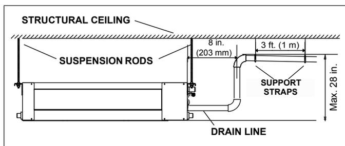
Figure 12. Condensate Drain with Factory Condensate Pump
